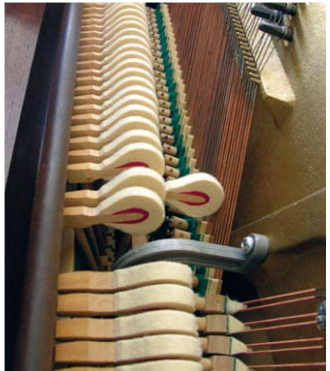
Example of traditional use of felt in piano.
